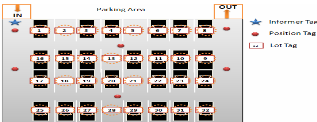
Fig. 6. Illustrate the setup for supporting navigation towards the reserved or idling parking lot
