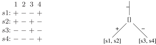
Fig. 1. Left: An example data of four sequences ( s_1, s_2, s_3 and s_4 ) of length 4 over \Sigma = \{+, -\} . Right: A trie representation of the candidate set \mathcal{C}_2 = \{+-, --\} of the data on the left.
