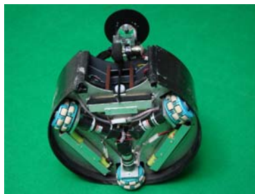
Fig. 2. Detail of the wheel configuration which enables an holonomic motion
