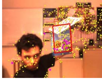
(b) Marked rectangle (in red): recognized object, SIFT features in dots (yellow), and SIFT features matched with the database in squares (purple).
