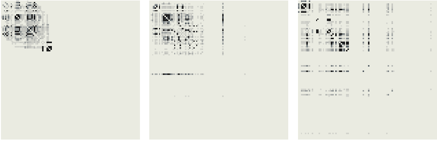
Fig. 2. Left: A minimized bandwidth adjacency matrix of a graph with 101 vertices. Middle and right: Two different permutations applied to the left matrix: The repair count measure quantifies the number and size of steps that are necessary to “repair” the matrices and result in the left one. The repair count of the matrix in the middle is smaller than the right one which meets intuitive user observations. Background color indicates 0, black represents values \geq 100 .
