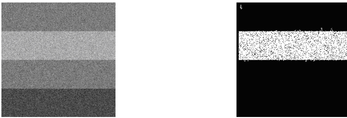
Fig. 5. Gaussian white noise field with extensive strip regions (on the left) and the result of segmentation with one-sided maximal likelihood threshold (on the right)
