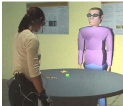
Fig. 3. Virtual agent Max with a human interaction partner standing around a table in a CAVE-like Virtual Reality environment. By means of his peripersonal space Max may perceive objects located on the table in front of him as near or far away from his body.
