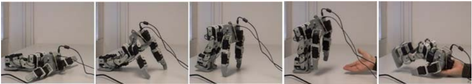
Fig. 3. Direct replay of a demonstrated standing up skill by the small humanoid robot. The robot fails to stand up, because of the missing support forces of the human teacher.
