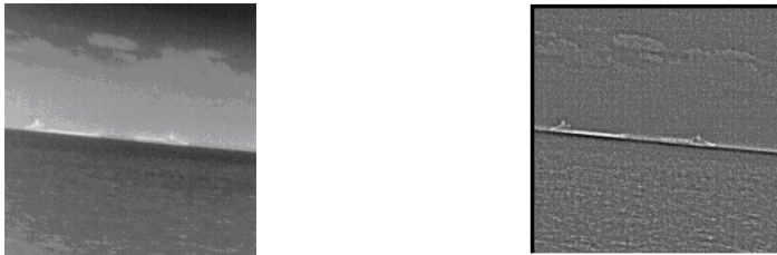
Fig. 1. The original infrared image of two ships on sea and pre-filtered image with the use of sample average in 9x9 window
