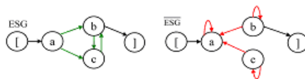
Fig. 1. An event sequence graph ESG and \overline{ESG} as the complement of the given ESG
