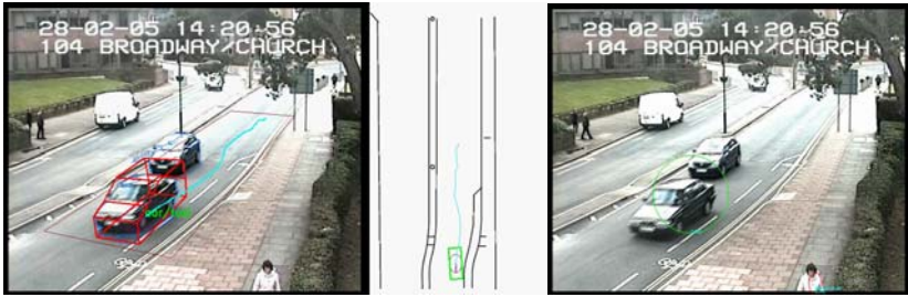
Fig. 4. The second car is missed due to occlusion between the vehicles. The proposed classifier on the left correctly locates the first car. The OpenCV tracker merged both cars with a large bounding box at a central position.
