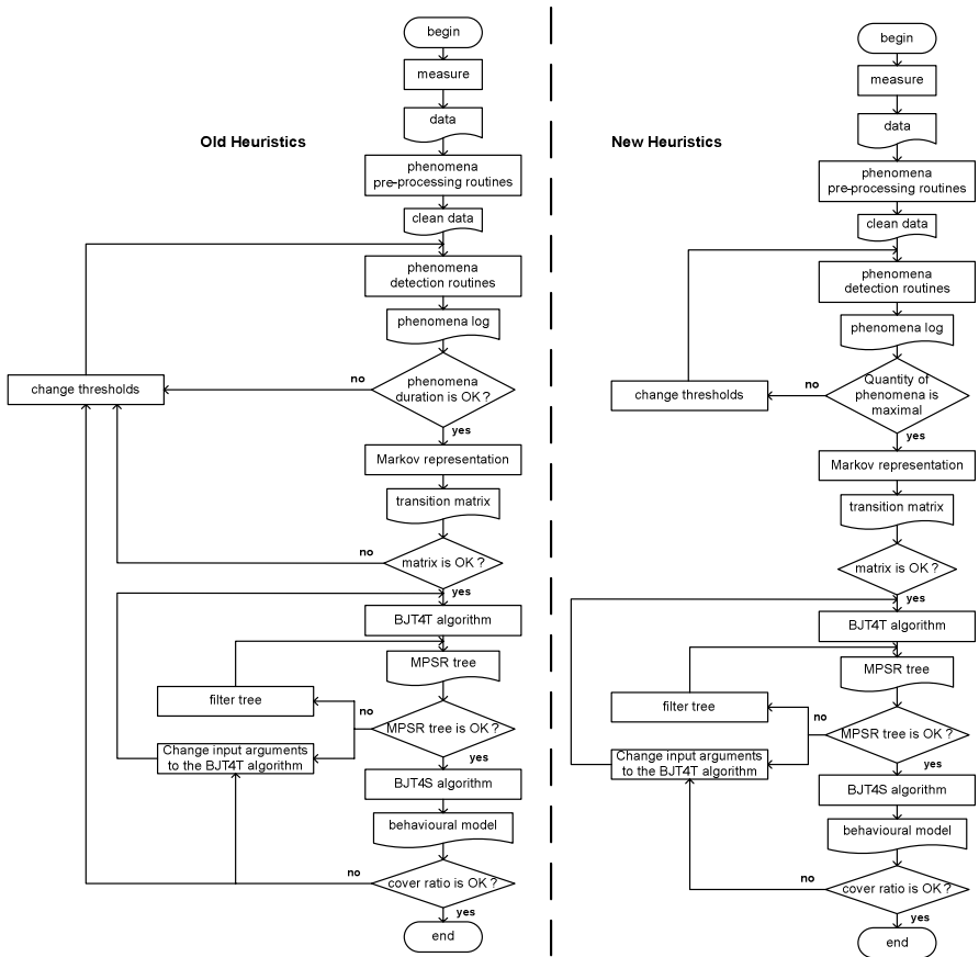
Fig. 3. Comparison of the two heuristics. Notice that several feedback links have disappeared.
