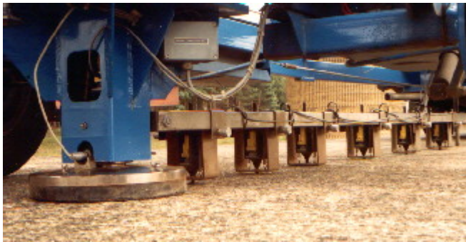
Fig. 5. FWD Application ( http://training.ce.washington.edu/wsdot/ )
