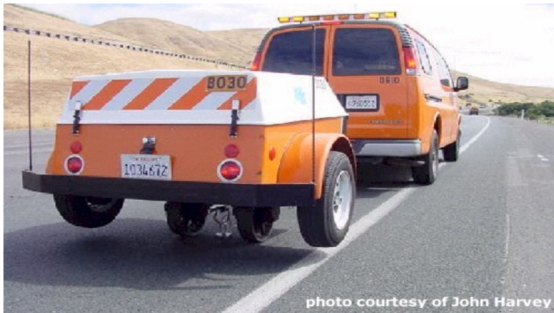
Fig. 4. Dynaflect in use ( http://training.ce.washington.edu/wsdot/ )
