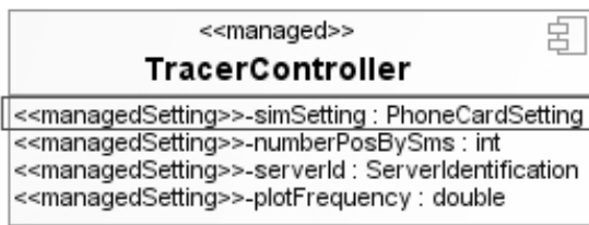
Fig. 3. A Managed Component of the Tracer Subsystem
