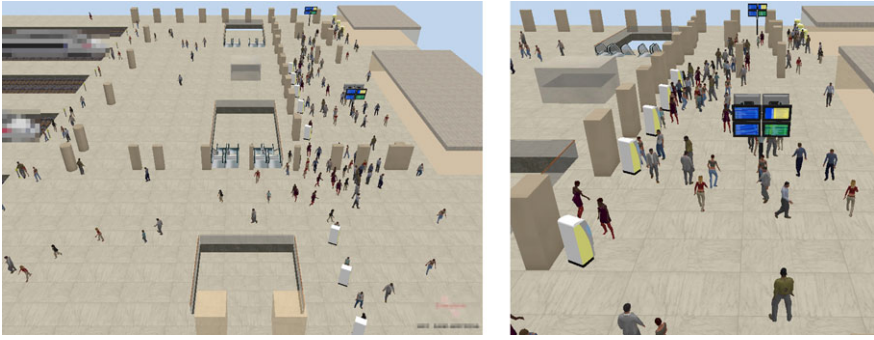
Fig. 10. Crowd simulation of a real case: Gare de Lyon in Paris . All agents are fully autonomous with individual behaviours.
