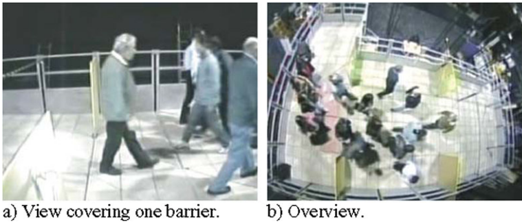
Fig. 2. CCTV cameras were set up monitoring each barrier, with two further cameras giving platform overviews.
