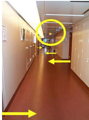
Fig. 11. Architectural space vs. escape signage.
