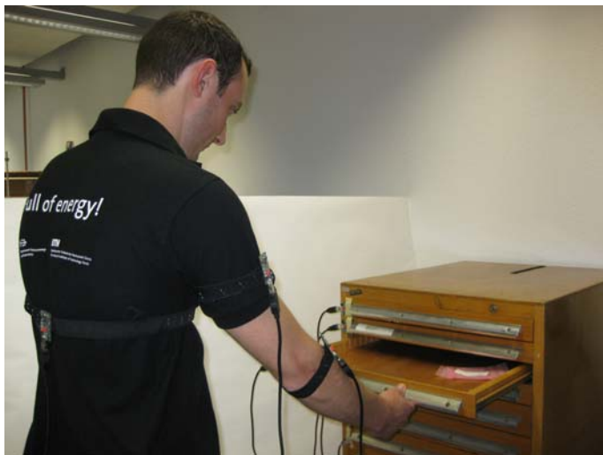
Fig. 2. Experimental setup: drawers equipped with sensors playing the role of Ambient Cells and sensors on the body of the user playing the role of the Wearable Cells
