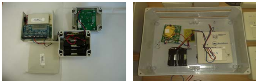
Fig. 1. IPSensor node with attached CO 2 sensor is shown on the left and the weather-proof box is shown on the right
