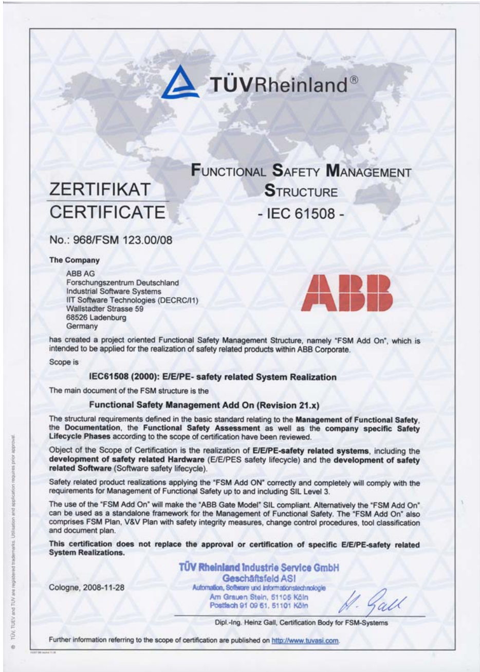
Fig. 5. Certificate of compliance of the FSM Add-on with the requirements of IEC 61508 up to and including SIL 3
