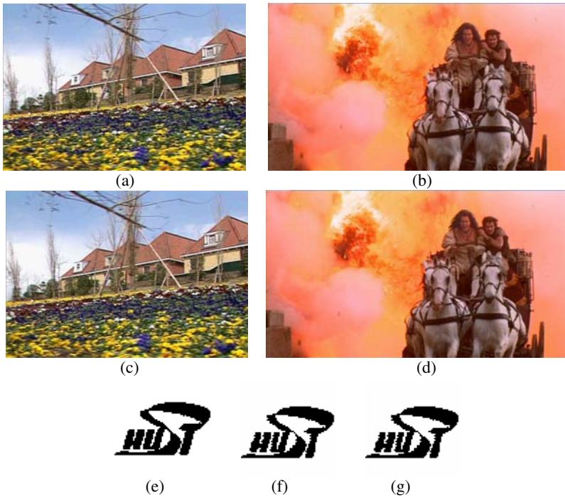
Fig. 2. Host video and watermark (a) Original video Flowergarden (6Mbit/s) (b) Original video Cutthroat (8Mbit/s) (c) Watermarked video Flowergarden (d) Watermarked video Cutthroat (e) Original watermark (f) Watermark extracted from Flowergarden (g) Watermark extracted from Cutthroat
