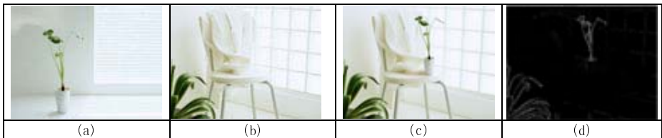
Fig. 3. One of the false experiment results. (a) and (b) are two original images; (c) is a forgery by moving the plant from (a) to (b) and using feather operations. (d) is the experimental results of (c) using the method in this paper, and the traces of feather operation are marked by white points.
