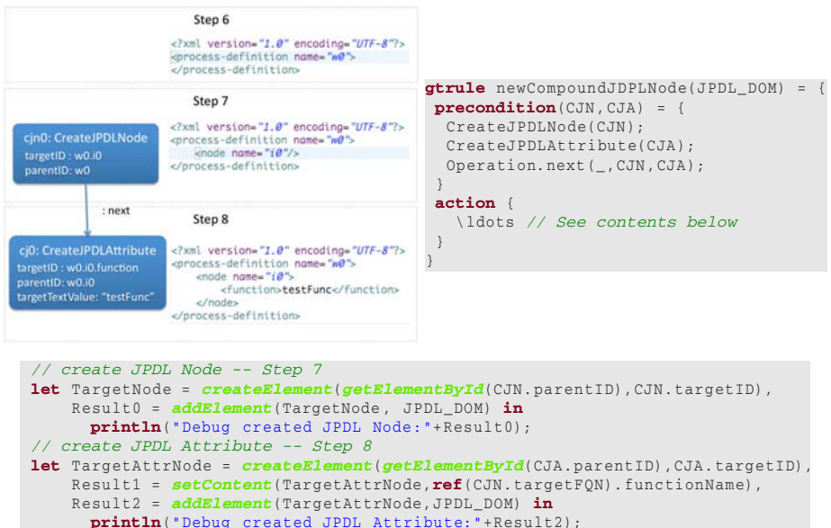
Fig. 8. Applying CHMs through the jPDL XML-DOM API
