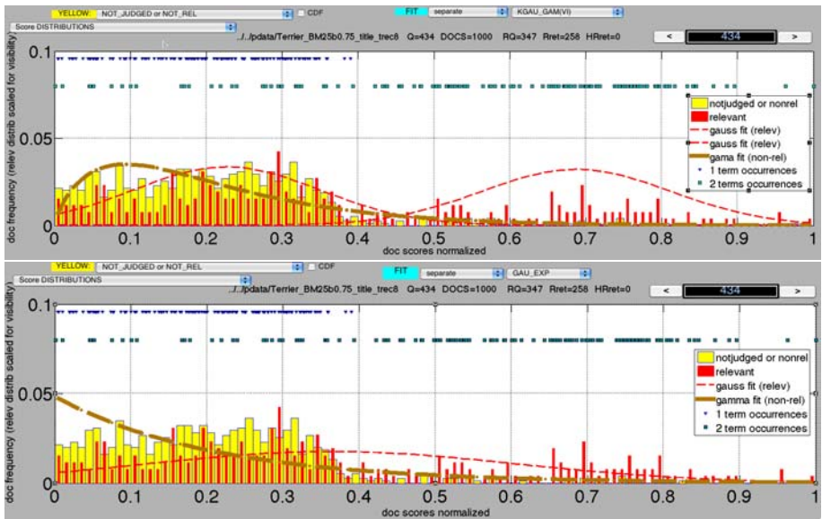
Fig. 1. The histogram over the scores of non-relevant and relevant documents and the Gamma and k Gaussians distribution (top) along with the negative exponential and single Gaussian distributions (bottom) fit into these scores separately
