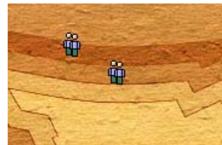
Fig. 4. Floor interface. Darker edges indicate a lower floor. In this case, two people are located on the ground floor and two more are located on the first floor.
