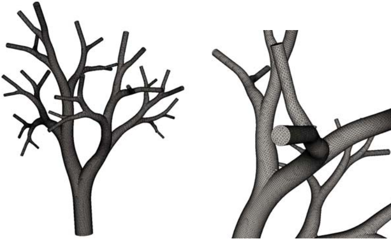
Fig. 16. A mesh of a 6 generation airway of a human lung. The mesh on the right is a close-up view showing the sharp curves generated at the end caps of the model. (Model provided courtesy of Kwai Lam Wong, Oakridge National Laboratories.)
