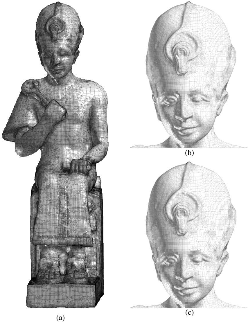
Fig. 5. Hexahedral mesh for a Ramses model (a-b) using the new set of the refinement templates (2.14M elements) and (c) the previous set (2.20M elements)
