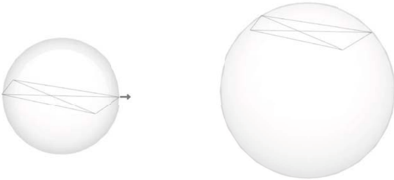
Fig. 3. Circumsphere of a sliver. Before perturbation (left), the sliver is close to the equatorial plane of its circumsphere. A very mild perturbation of one of the sliver vertices (right) makes its circumradius increase considerably.
