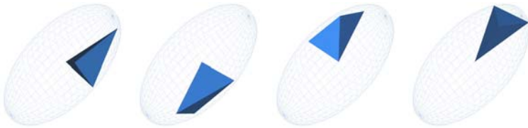
Fig. 1. Some unit-elements with respect to a 3D metric represented by its unit-ball.
