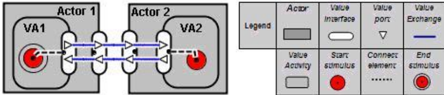
Fig. 1. Basic e3-value constructs
