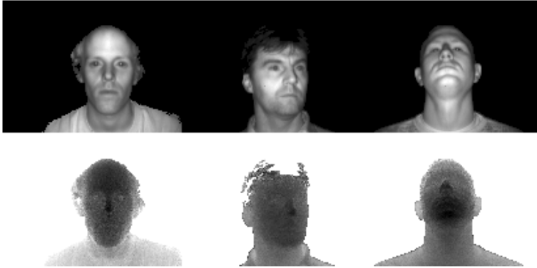
Fig. 1. Three sample images of frontal face images taken by an SR3000 TOF camera. The top row shows the intensity and the bottom row the range data.
