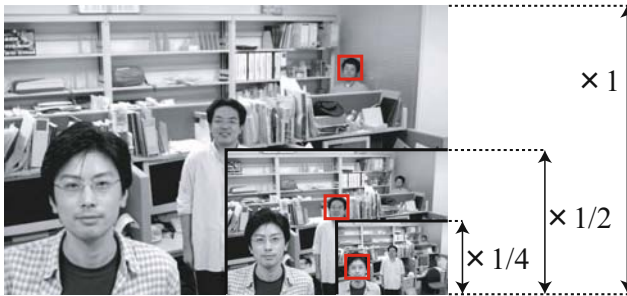
Fig. 1. Concept of multi-resolution image perception. Any size facial images can be detected by combination of (1/2)^n -scaling of input images and use of three template image sizes of 100%, 80%, and 60%.
