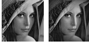
Fig. 3. Left: Original image. Right: Approximation obtained through the DC component of Eq. (7), computed over 3 \times 3 windows. Representation error of 6.6%.
