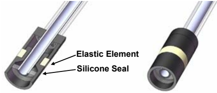
Fig. 3. A 14 gauge needle passes through the sensor to deploy surgical anchors
