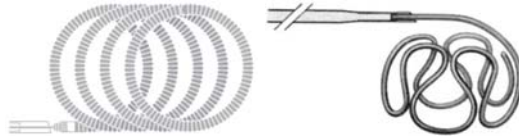
Fig. 1. Example of coils used in our simulations, left: Boston Scientific helical coil GDC 10, right: 3D GDC built with omega loops [13]
