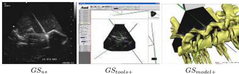
Fig. 1. The three guidance systems evaluated. The virtual needle tool also has x,y and z axis extensions with 10mm markers to help locate the tip and its trajectory.
