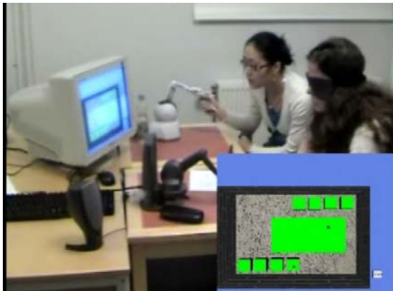
Fig. 2. Haptic collaborative application in which both users can pick up and move around objects (small picture in picture). Two users are seen using one haptic feedback device each.
