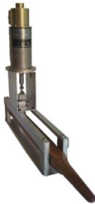
Fig. 6. The haptic carillon single-baton prototype
