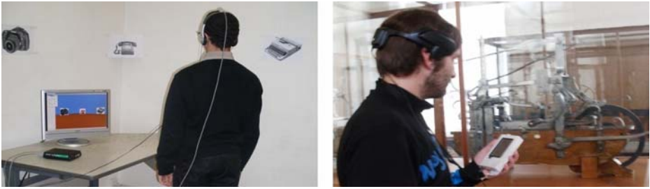
Fig. 2. (Left): User holding the PP sensor, looking towards the objects of the real scene; his field of vision is reproduced on the interface. (Right): Experimenting with the PERCIPIO headset at the CNAM museum.
