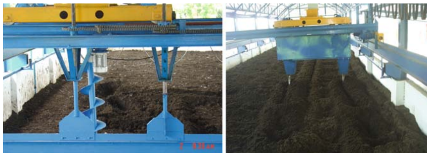
Fig. 15.1 The organic fertilizer pilot plant production with two sets of ribbon screws
