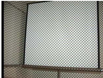
Fig. 5. An example of checker flag pattern used in the “Separation of Direct Component and Global Component” method
