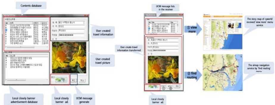
Fig. 7. The example of the UCM message authoring tool (left) and the UCM message decoding tool and the implementation by PC internet service (right) [13]
