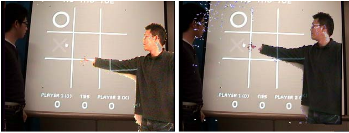
Fig. 8. Synthesized images. The left image is synthesized by conventional photometric calibration without geometric calibration. The right image is synthesized by proposed method.
