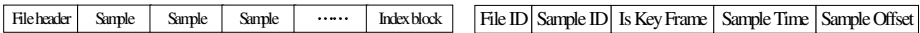
Fig. 1. File format structure of AVI video and the formed temporal indexing structure
