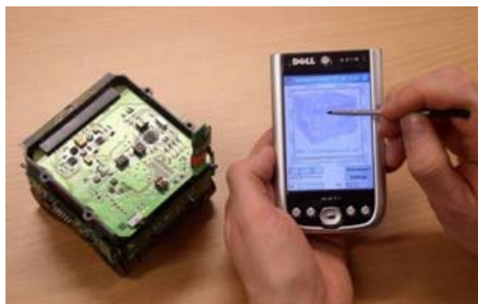
Fig. 4. Remote control of the robot via a PDA
