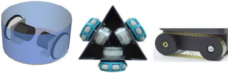
Fig. 3. Evaluated drive systems: differential drive, omni drive and chain drive
