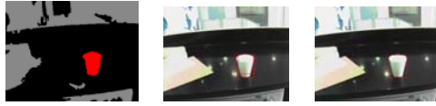
Fig. 3. An example of cup detection. The images from the left to right are: color-based segmentation, HOG-based detection, final detection by fusion.
