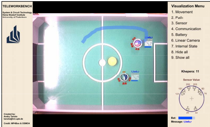
Fig. 8. Robot soccer (here KheperaSot setup) on the Teleworkbench platform. The robots can be programmed via the Internet. Matches can be started and monitored online via a web browser as well as recorded for detailed match analysis.
