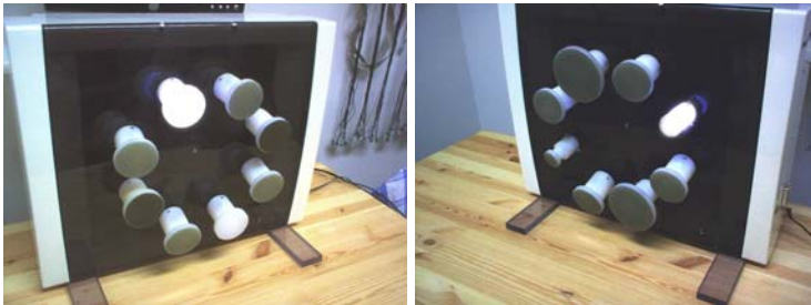
Fig. 2. Movement Execution Device (MED). Simple action context (A) consisting in objects that vary along the luminance dimension (LED lighting up and the objects on MED are all defined by luminance) and complex action context (B) consisting in objects that vary along the luminance dimension (LED lighting up) and size dimension (items on MED).
