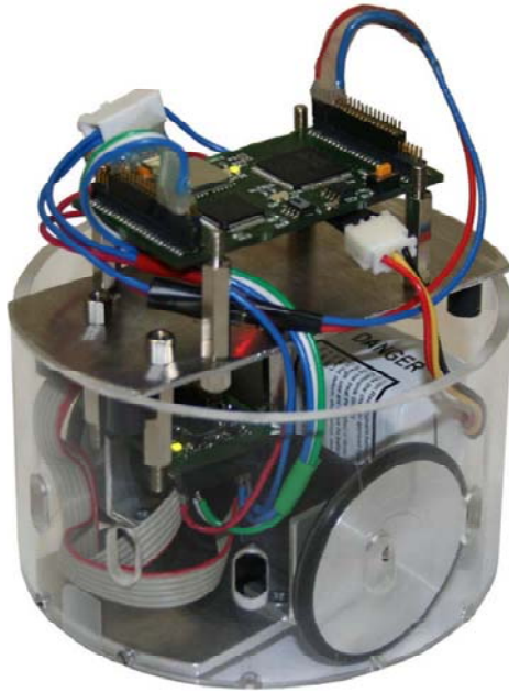
Fig. 2. Prototype chassis of the AMiRESot robot (shown electronics is used for testing only, final version will be different)
