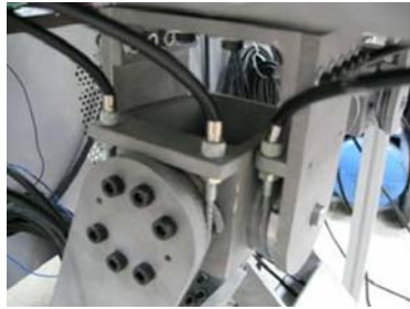
Fig. 4. Photo of realized hip module in an AK leg mechanism
