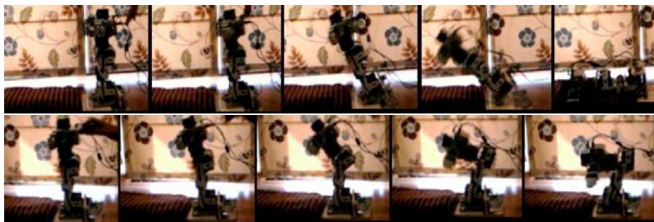
Fig. 6. Response of Bioloid to a disturbance of 1N. The stiff robot in (top) falls down. The reflex-endowed robot in (bottom) absorbs the disturbance.
