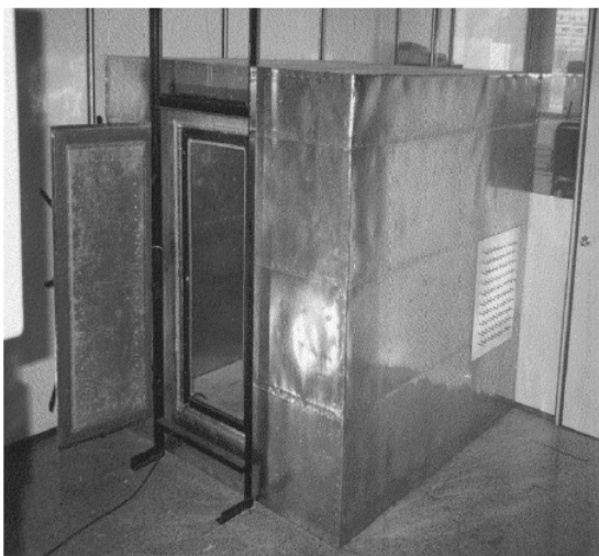
Fig. 2 Anechoic chamber developed for electromagnetic radiation tests. Dimensions were width=2.0 m, length=2.0 m and height=1.9 m. The inner walls of the cage were made of steel and the outer walls were made of copper.
