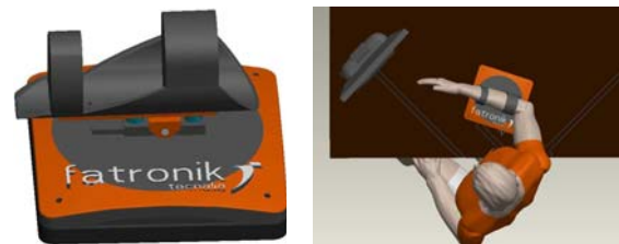
Figure 1. The ARMassist (left) is a wireless human interface device that connects to the user forearm and is operated on a standard table (right).
