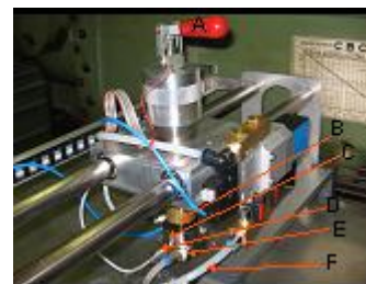
Fig. 2 Pneumatic test device A: the lever; B: the brass piston (containing the spring); C: the load cell; D: the pressure transducer; E: the stainless steel element (around the pressure chamber); F: the pipe from the valves (connected in parallel).
