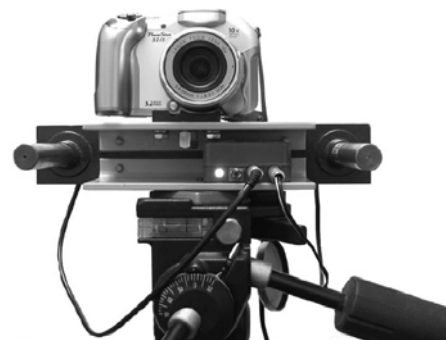
Fig. 2 Tripod with camera and laser collimator
