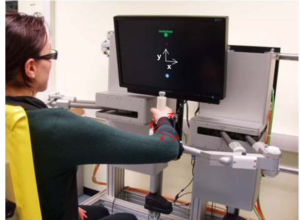
Fig. 1. Subject performing horizontal arm movements with/without lateral constraint using the Braccio di Ferro workstation.
