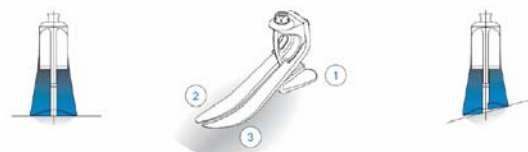
Fig. 2 Elite Foot prosthesis: 1, 2, 3 – components which are fabricated from composite materials like carbon fiber
