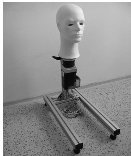
Fig. 5 Model of the head and stepper motor including planet gearbox (verification of rotation measurement)
