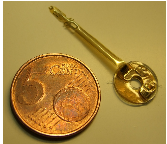
Fig. 2 The fully implantable epiretinal EpiRet retina implant. The implant can be telemetrically activated and has 25 electrodes (top side). Each metal-oxide electrode has a three-dimensional shape and was electrically activated and tested. However, this ensures excellent stimulation results. On the right side of the picture are the receiver coil and the electronics protected by parylene C against moisture (ions) and embedded in silicone rubber. Note the picots required for thread-fixation in the eye's lens-capsule. The five-cent coin serves as a ruler.
