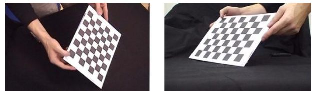
Fig. 1: Calibration images from two different cameras containing the chessboard.
