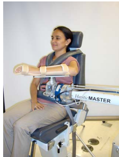
Figure 1. Measurement of work area with the ACT 3D robot.
