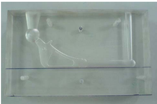
Fig. 5, Finished die half (1 side) after polishing.
