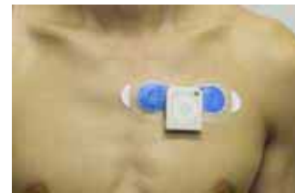
Fig. 1 IC chipped 3 axes accelerometer combined ECG on the sternum
