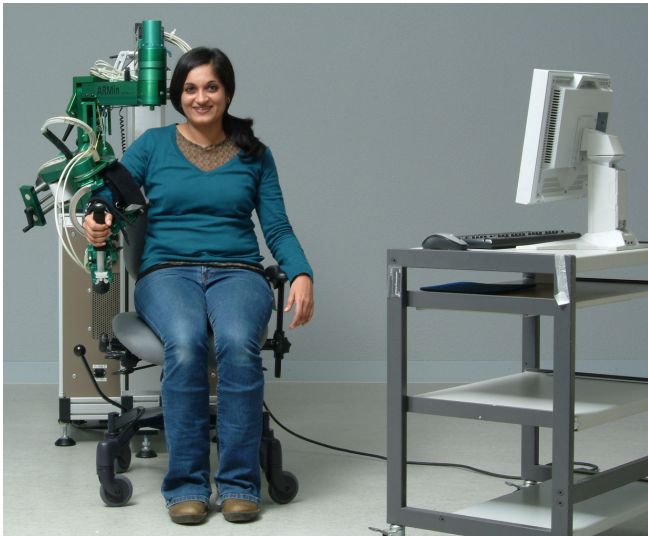
Fig. 1: ARMin III exoskeleton robot with a healthy subject. The device has six actuated DoF and connects to the most affected arm. A computer monitor shows different graphical scenarios to the patient.
