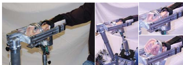
Figure 3: HapticDrive device prototype for arm and wrist training
