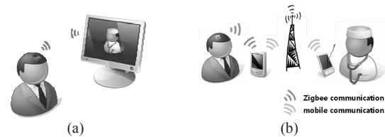
Fig 3 A remote rehabilitation service for stroke recovery using a ZigBee-based neuro-modulation system. The patient's IPG is connected to doctors at a remote site through a) the internet and PC, b) a mobile network and various handheld devices.
