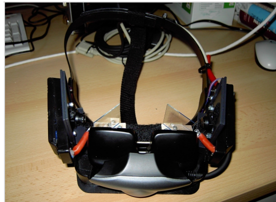
Fig. 4 Displays units - specialized glasses with eMagin 3DVisor®
