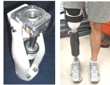
Fig. 3 Knee prosthesis mechanism without carbon fiber coating (left) and final knee prosthesis adapted to a user (right)
