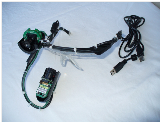
Fig. 5 The eye tracker unit with the measurement cameras
