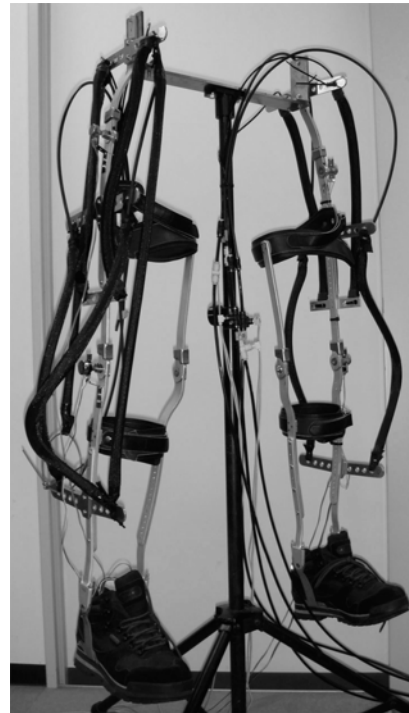
Fig.3 provides an overview of the gait training orthosis. We had suspended the orthosis on an experimental frame.
