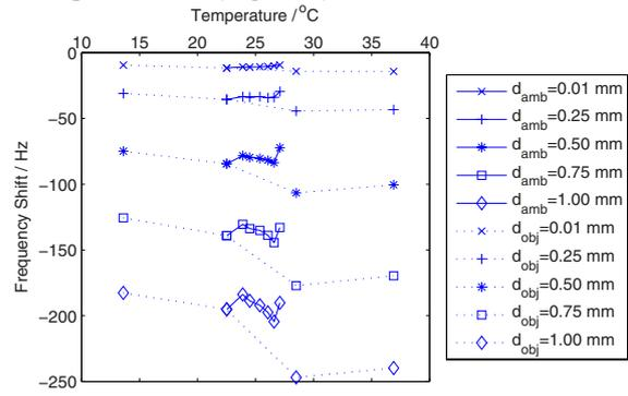
Figure 3 Frequency shift at various impression depths: Straight lines when ambient temperature was varied; dotted lines for varied rubber silicone plate temperature spanning from refrigerated to normal body temperature.
