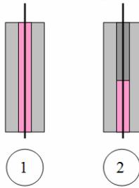
Figure 1 Steel pipes molded into cylindrical RSE with: 1) Full amount of filler material. 2) Half amount of filler material.
