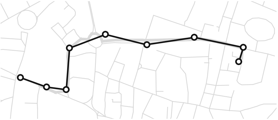
Fig. 2. Sample GPS trace (black) and the path as attached to the topological base map data (thick gray). This example uses OpenStreetMap data rather than the OS ITN layer used for the actual experiments.
