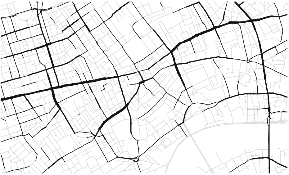
Fig. 5. Space syntax measures of the central London area (angular betweenness radius 1.5km). At this radius, which reflects local journeys, the inner London ring road (part of which is visible in the top left corner) is not highlighted. (Map data: OpenStreetmap).
