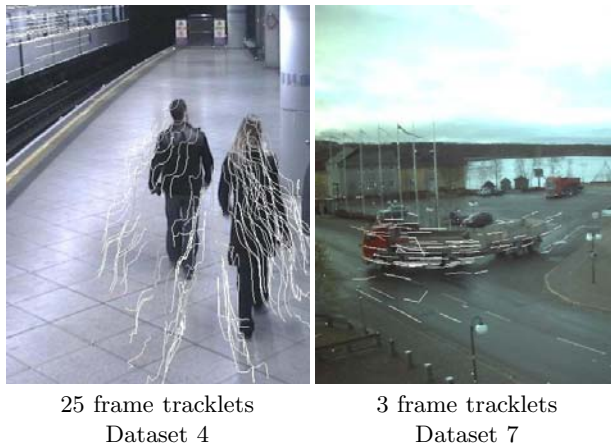
Fig. 1. Single frame of video showing tracklets: these give a robust indication of motion in the image plane without committing to any object segmentation or scale
