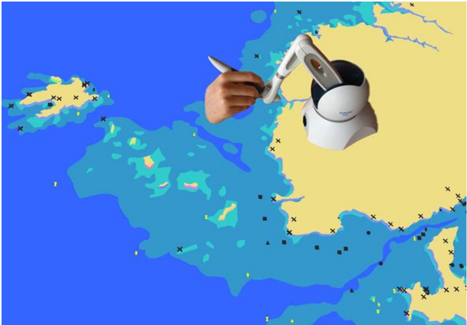
Fig. 1. A visualization of the SeaTouch virtual maritime environment. A participant’s hand is interacting with the stylus of the Phantom haptic mouse. The land area, coastline, and maritime features are displayed.
