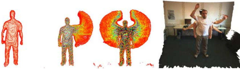
Fig. 8. Left: Accumulated hitcount for video sequence over time, color coded: red ( < 60 ) - black ( \geq 360 ). From left to right: Frame 1; Integration of frame 1 to 120; integration of frame 1 to 375. Right: Rendering by selection of 3 time frames of the Space-Time Video.
