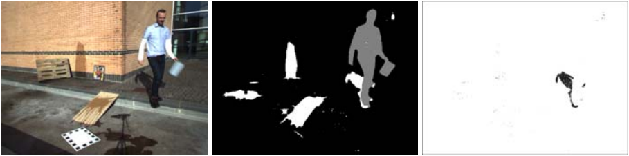
Fig. 2. Processing results from frame 137 out of a recorded sequence of 200 frames. Left: The current frame where the person has entered the scene and has splashed water from the bucket onto several surfaces in the scene. Middle: result from background subtraction, segmented into foreground object (grey) and shadow candidate pixels (white), which include all the detected water splashes since the water has caused the surfaces to change appearance. Left: pixels identified as being in shadow after chromaticity analysis. Note that the shadow cast by the camera tripod is a static shadow, and as such is not detected by the presented approach.
