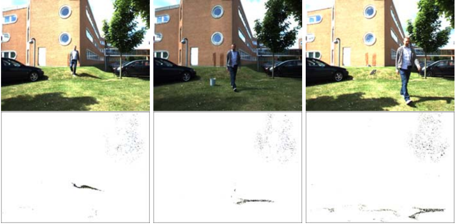
Fig. 9. Dynamic shadow detection based on image differencing (frames 180, 520, and 1741).
