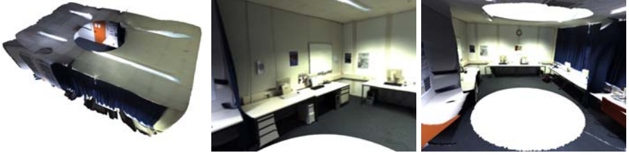
Fig. 4. Triangle mesh generated from 2.5D panoramic image. Top Left: View of complete environment model. Others: Three views of the interior.
