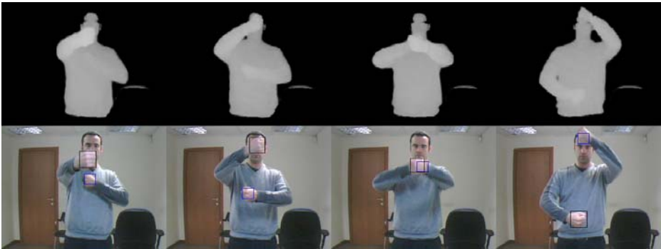
Fig. 5. Tracking a sequence with occlusions (a) initial tracking window is intentionally placed close to the body on left hand to make the tracking harder as variance is low in the depth image in that window (b) hand is occluding the face, both having a similar color histogram. Tracking works well with additional depth data, but stays on face when relying on color only. (c) hands completely occlude each other but continue to track well afterwards when depth information is added to the histograms. (d) tracking continues successfully even when close to body, a case in which tracking based on depth only will fail.
