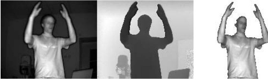
Fig. 1. Sample image taken with a MESA SR4000 TOF camera. The leftmost image shows the amplitude data. The range image is given in the center and the resulting segmentation is shown on the right.
