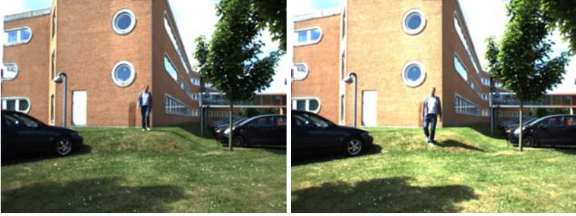
Fig. 8. In partly overcast, windy conditions illumination changes can be drastic. These two frames are 15 frames apart, corresponding to a time difference of 1.5 second. On average the latter image is 50% brighter than the former.
