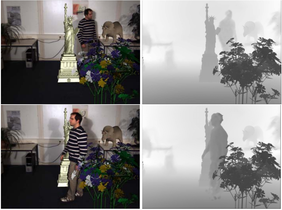
Fig. 5. Color and depth mixing for a frame of an input sequence. Left: Original image of person walking, augmented by virtual objects with mutual occlusion. Right: corresponding depth map used for mixing.
