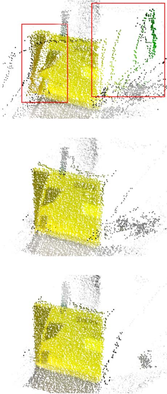
Fig. 6. Scene 1 before (top) and after motion compensation (middle) as well as the static reference scene (bottom). Note the motion artifacts due to texture changes of the box surface.
