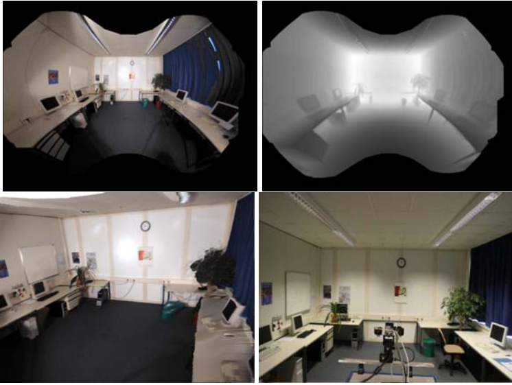
Fig. 3. 3D Panorama of the environment (top row: color and depth) with rendered views of the resulting textured surface (bottom left). Bottom right is showing the position of the camera rig during the model generation.
