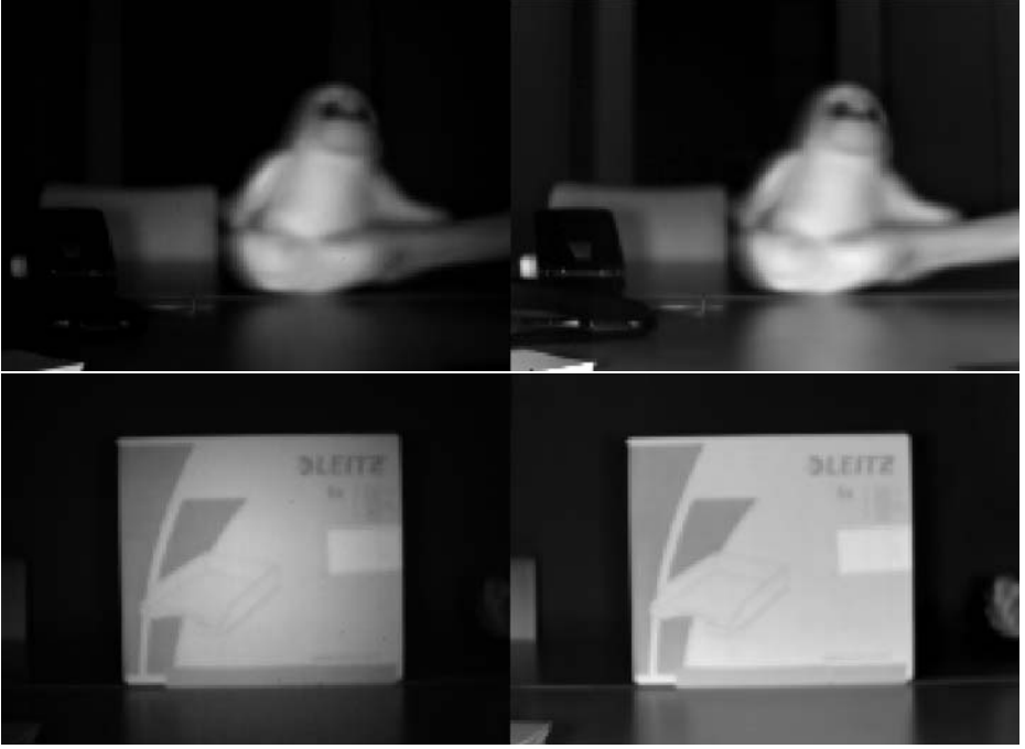
Fig. 3. PMD intensity image before (left) and after homogeneity adjustment (right). Note the strongly varying intensity of the hand/arm without correction.
