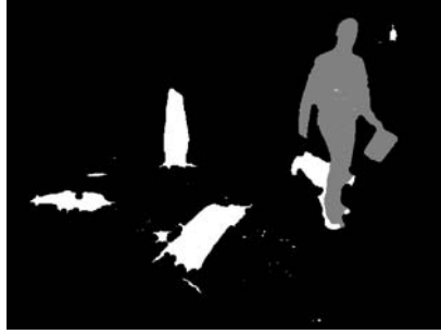
Fig. 4. Classification of pixels into foreground (grey), background (black) and shadow candidates (white)
