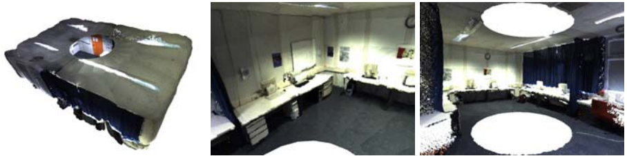
Fig. 5. Environment model as octree, fused from 115 images, cellsize 25mm^3 . A slight degradation due to point rendering is visible.
