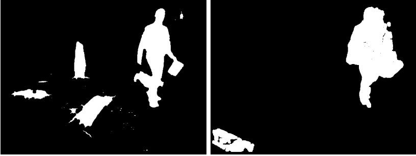
Fig. 3. Left: Pixels (frame 137) determined by the Codebook method as being different from the trained color background model. Right: Pixels (also frame 137) determined as being different from the disparity background model.
