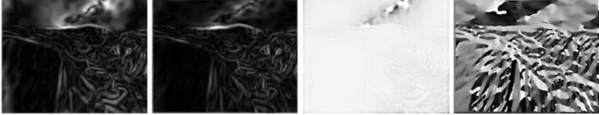
Fig. 5. The 3D conformal signal delivers four local features which can be used for image sequence analysis such as optical flow and motion analysis. From left to right: Curvature, phase and the two parts of the orientation information. 3D convolution mask size 5 \times 5 \times 5 pixels.
