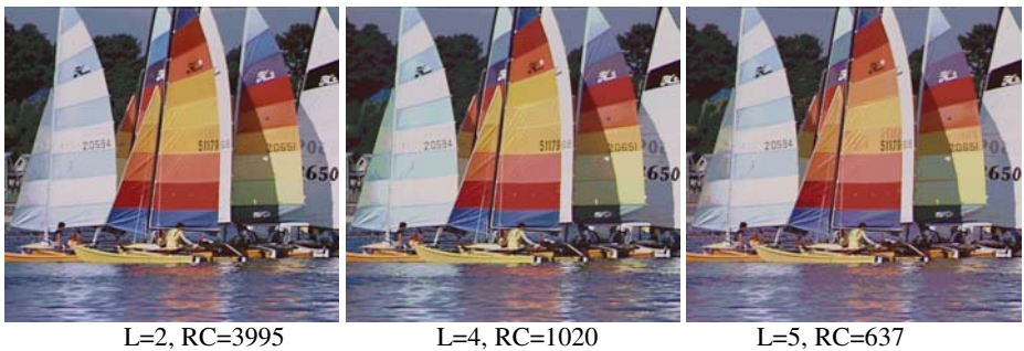
Fig. 3. Quantized images resulting for different values of L . In all cases, the number RC of representative colors is considerably smaller than the number OC of original colors ( OC=150053 )
