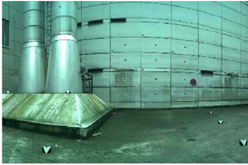
Fig. 4. Left: calibration marks are distributed around a courtyard at TFH Berlin. Right: deviations between calculated image coordinates and their actual reference coordinates in this courtyard (listed values in subpixels).
