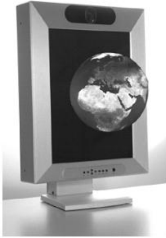
Fig. 10. Auto-stereoscopic display made by Fraunhofer HHI
