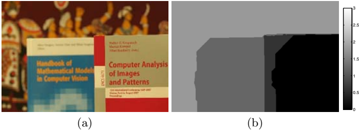
Fig. 1. The depth recovery result of the book image. (a) The input defocused image. (b) Recovered layered depth map. The larger intensity means larger blur amount and depth in all the depth maps presented in this paper.
