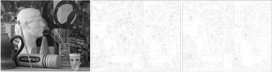
Fig. 4. Left: Art image that has been smoothed. Centre and Right: difference image between LUT and fast-trilateral filter, using \varepsilon = 10^{-4} (centre, \max(d) = 0.36 ) and \varepsilon = 10^{-12} (right, \max(d) = 3.1 \times 10^{-5} ), with \sigma_1 = 9 . Difference images scaled for visibility, white \leftrightarrow black into 0 \leftrightarrow \max(d) .
