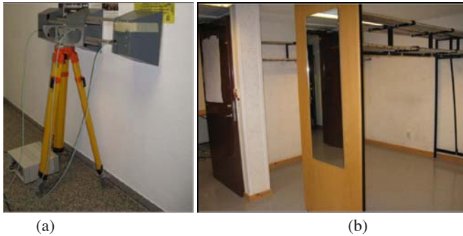
Fig. 2. (a) Experimental M-sequence UWB radar system, (b) Measurement room interior
