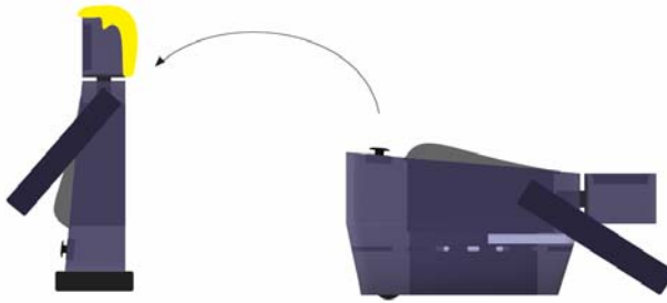
Fig. 5. Basic design of the IROMECE robot in vertical and horizontal configuration
