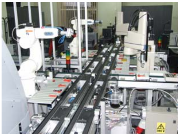
Fig. 7. Layout of the manufacturing cell with holonic control
