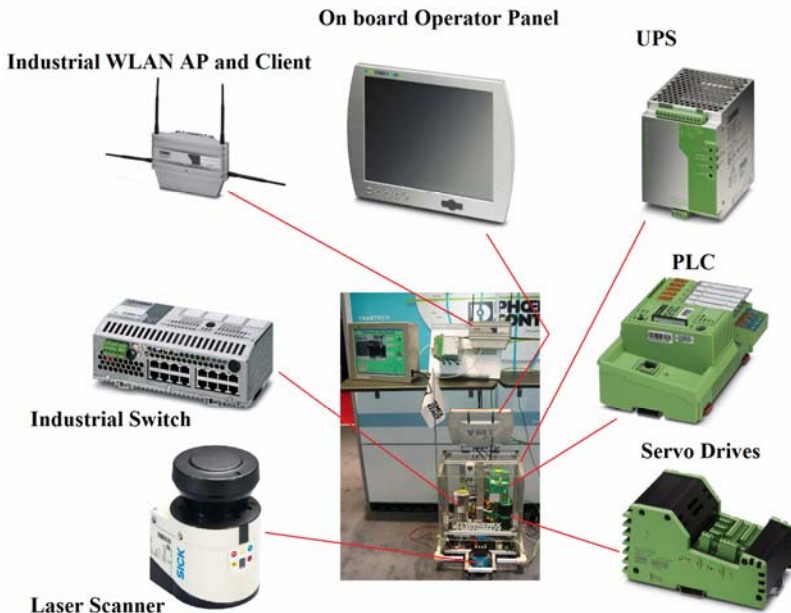
Fig. 7. The accomplished system with the main components
