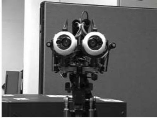
Fig. 5. The humanoid robot head with stereovision
