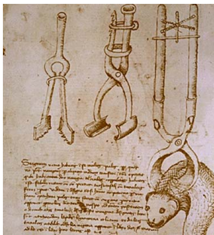
Fig. 6. A variety of two-finger grippers with different locking systems for fish grasping by Mariano Di Jacopo in 14 th Century
