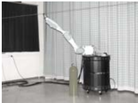
Fig. 6. A combination of a mobile platform and a robot manipulator
