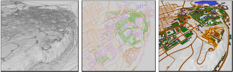
(a) Triangulated elevation (3D). (b) Merged semantics (2D). (c) Fused map (3D).
