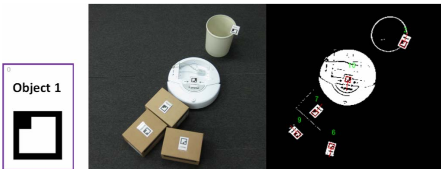
Fig. 6. Vision-based ID Tag and Tracking Results
