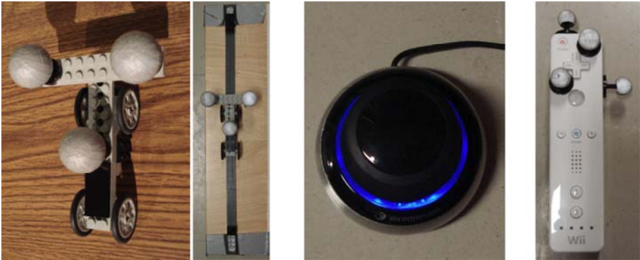
Fig. 1. The devices (mouse not shown). From left to right: the DepthSlider alone and on its rail, the SpaceNavigator TM , and the free-space device Wii Remote TM tracked by a Vicon TM .
