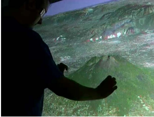
Fig. 1. A user interacting with an interscopic multi-touch surface (iMUTS) in a landscape planning scenario in which depth cues are important, e. g., in a landslide risk management scenario. The geospatial data is displayed in anaglyph stereoscopic mode.
