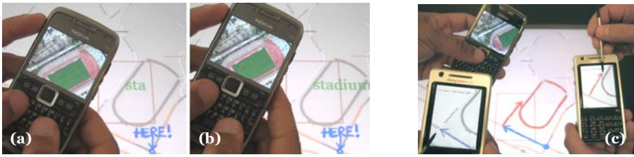
Fig. 2. a–b) The lack of tactile buttons on the surface can be addressed by using the physical keyboard of the mobile device. Here, the user enters “Stadium” on a point of interest. c) Simultaneous input from multiple uniquely identified devices allows collaborative scenarios. A blue arrow has been drawn on the left device, while a red arrow and an outline of the stadium has been added using the right device.
