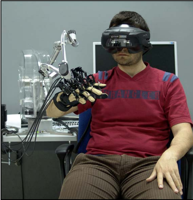
Fig. 5. Direct first-person hand interaction in the proposed virtual maintenance application using the CyberForce force feedback system
