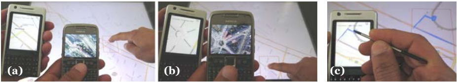
Fig. 1. a–b) Multiple mobile devices are wirelessly connected to the surface and provide individual visualizations (road maps and satellite images) of the region indicated by the user's touch. c) The higher input resolution of the mobile device's touch screen allows the user to create precise annotations, while also being able to work in a comfortable pose.
