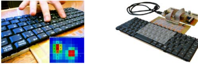
Fig. 1. Left: Color value map and finger position on the keyboard. Right: DGTS electronics.
