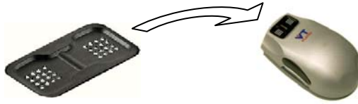
Fig. 1. VTPlayer mouse, with two 4x4 pins matrices on the top
