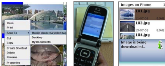
Fig. 1. Downloading a picture from the laptop to the mobile phone with Touch & Connect: select the appropriate option for a picture and touch the tag on the laptop with the phone
