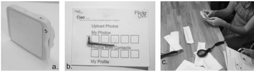
Fig. 2. Lowest level prototype: a) the foam model, b) a paper screen c) the trial set up
