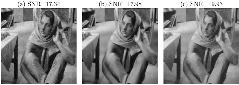
Fig. 5. Comparison with other methods. Denoising of image f from Fig. 4. (a) TV-denoising ( \lambda is chosen to achieve the best SNR, \lambda = 0.1 ), (b) Translation Invariant Wavelet Denoising (the threshold is chosen to achieve the best SNR) and (c) our result which achieves a better SNR.
