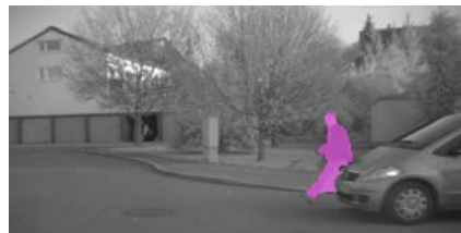
Fig. 9. The figure shows the energy images and the segmentation results for objects which move not parallel to the camera motion. In such constallations a monocular as well as a binocular segmentation approach is successfull. However, one can see in the energy images and in the more accurate segmentation results (the head of the person in the Running sequence) that stereo is more discriminative. Note, that the also non-rigid independently moving objects are segmented.
