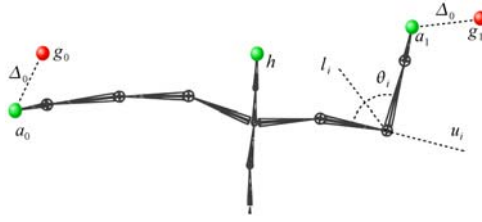
Fig. 1. An illustration of the kinematic model. End-effector positions are shown as green dots, while the desired positions (goals) are shown as red dots.
