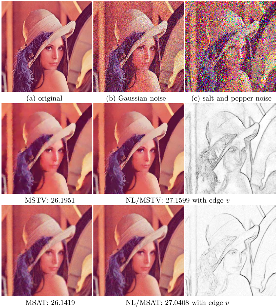
Fig. 1. Recovery of noisy image f = u + n and PSNR values. Top row: (a) original, (b) noisy image with Gaussian noise with \sigma_n = 0.02 , (c) noisy image with salt-and-pepper noise with noise density d = 0.3 . Middle row: recovered images of (b) and edge set v using MSTV: \beta = 0.17 , NL/MSTV: \beta = 0.07 . Bottom row: recovered images of (c) and edge set v using MSAT: \beta = 6 , NL/MSAT: \beta = 1.8 .
