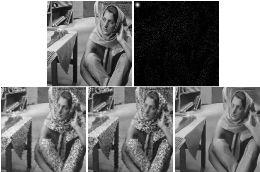
(b) Barbara , 512 \times 512 with 5% of the samples. 2nd line are results of: linear interpolation (PSNR 20.1), Laplacian interpolation (PSNR 19.9) and algorithm O with h = 100 (PSNR 22.8).
