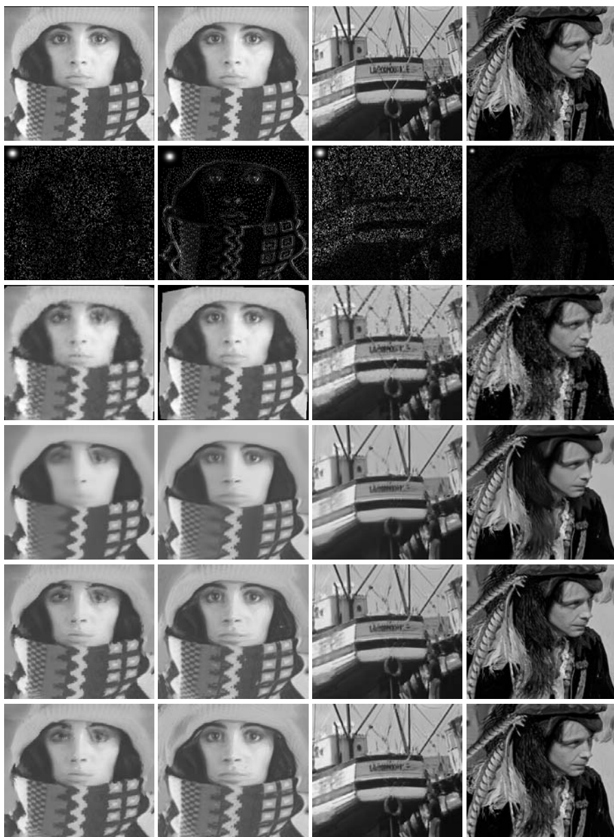
Fig. 3. Sparse sampling interpolation. 1st row: original images. 2nd row: input data with sample densities of 10%, 10% dithered [22], 20% and 9%. 3rd row: linear interpolation over the Delaunay triangulation of the samples; PSNRs: 25.8, 30.6 (not considering the black frame), 25.0 and 22.74. 4th row: results of method AB with h = 100 ; PSNRs: 22.5, 22.7, 25.5 and 22.79. 5th row: results of AB with h \rightarrow 0 ; PSNRs: 22.6, 23.0, 25.5 and 22.56. 6th row: results of the method O with h \rightarrow 0 ; PSNRs: 22.6, 21.7, 25.1 and 22.69. (Details can be better appreciated by zooming on a computer screen)
