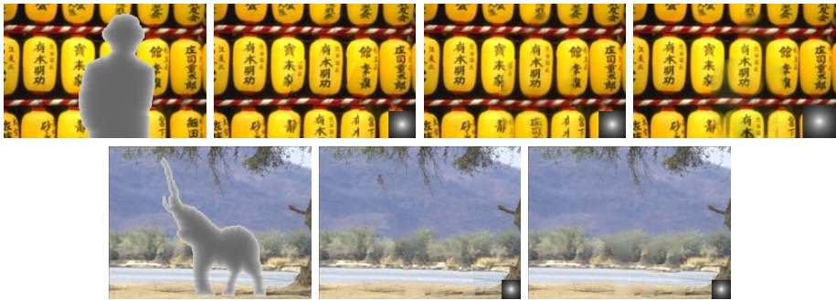
Fig. 4. From left to right, inpainting domain with confidence mask, result of path NL-medians, -means and -Poisson (the latter only for the first row). Top: cylinders - Results with s = 27 , a = 9 and h = 0 for patch NL-medians and -means and s = 33 , a = 1 and h = 0 patch NL-Poisson. Bottom: elephant - Results with s = 19 , a = 6 and h = 0 . The parameters of the confidence mask are \tau_0 = 5 and \kappa_0 = 0.4 in all cases except for the patch NL-medians with the bottom image, in which we set \kappa_0 = 0.1 . Results using RGB. Please refer to [17, 24] for other results on the same images.
