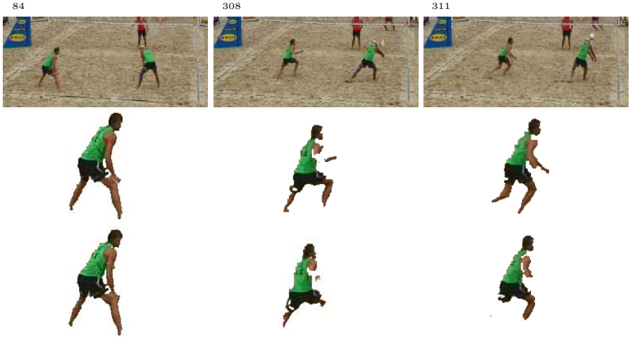
Fig. 2. Comparison of anisotropic TV and standard TV regularization. The first row shows frames of the original video where the left player is tracked. In the second row the anisotropic regularization term shows a better segmentation of fast moving details than the standard weighted TV regularization in the third row.
