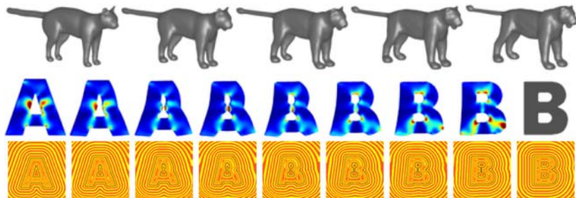
Fig. 1. Time-discrete geodesics between a cat and a lion and the letters A and B . Geodesic distance is measured on the basis of viscous dissipation inside the objects (color-coded in the middle row from blue, low dissipation, to red, high dissipation), which is induced by a pairwise 1-1 deformation map between consecutive shapes along the discrete geodesic path. Shapes are represented via level set functions, whose level lines are texture-coded in the bottom row for the 2D example.
