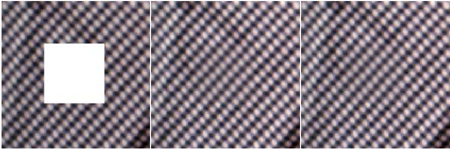
Fig. 8. Inpainting of 100 \times 100 size image with 40 \times 40 missing part. (left) data f , recovered using (middle) NL/MSAT: PSNR=35.6704, (right) NL/MSTV: PSNR=35.8024 ( 41 \times 41 search window, 9 \times 9 patch).
