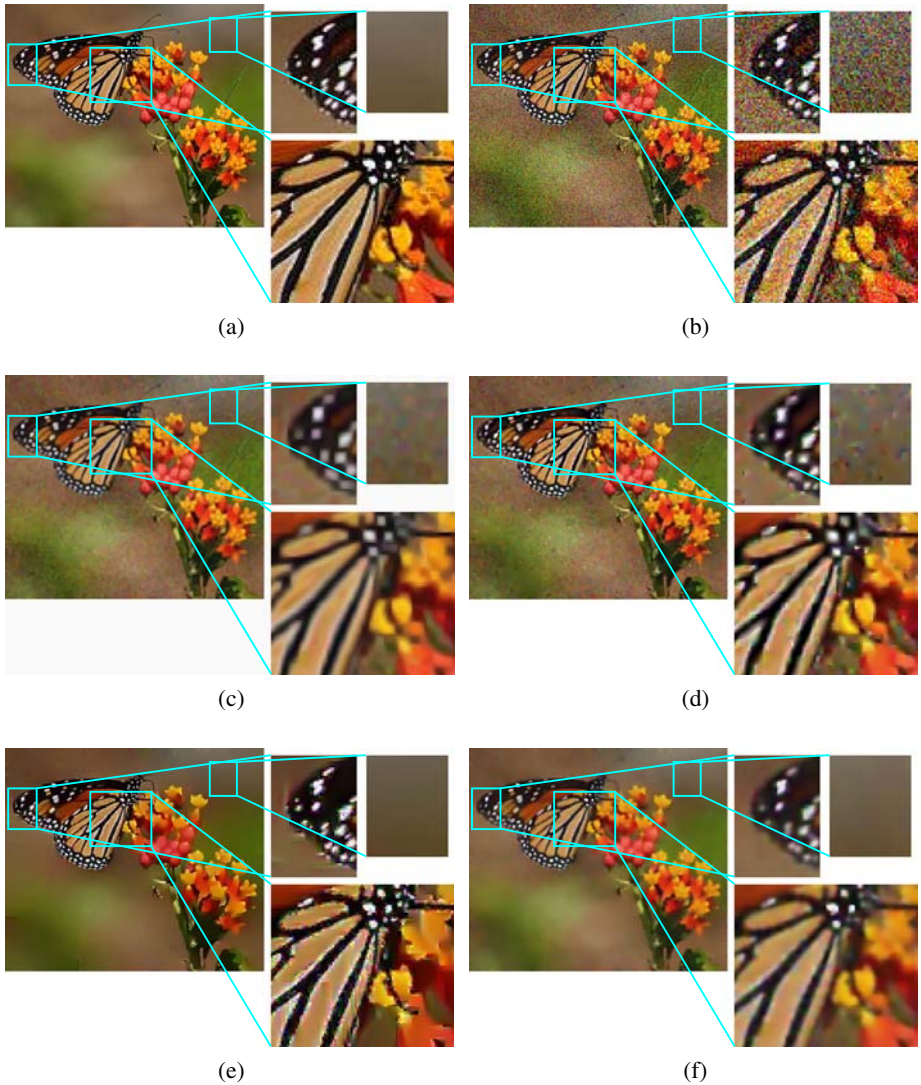
Fig. 4. (a) Original image. (b) Noisy image with a Gaussian noise of standard deviation 35. Denoised images using (c) the coherence enhancing diffusion, (d) the Beltrami flow, (e) the curvature preserving regularization, (f) our method.
