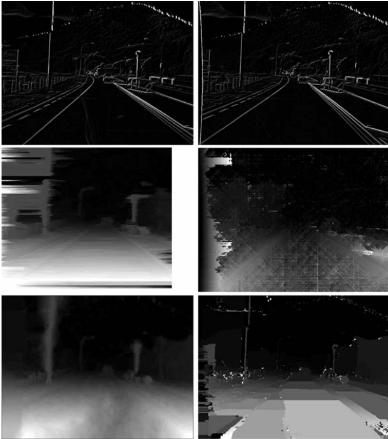
Fig. 4. Top: Sobel edge maps of the left-right stereo pair in Figure 1, used as stereo input pair. Middle: depth maps of single line DP (left) and Birchfield-Tomasi cost function in 8-ray DP (also known as SGM BT). Bottom: BP (left) and GC results.
