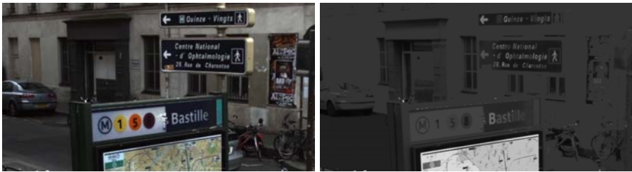
Fig. 2. On the left hand-side, an image, on the right hand-side the result (the transformation) of the ultimate height opening. Image copyright institut géographique national (IGN) .
