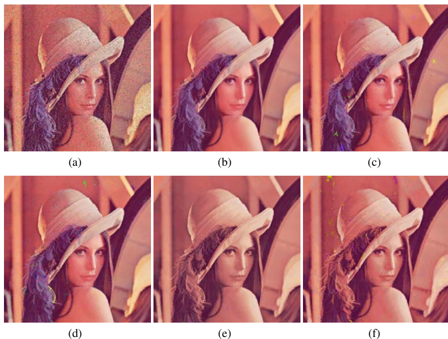
Fig. 2. Comparison of filtering operators \Psi based on area opening using different processing strategies. (a) Lenna image corrupted by 15% random noise. (b) Marginal processing ( M ). (c) Lexicographic ordering ( L ). (d) Distance-based total ordering ( dL ). (e) Preordering ( P_{mean} ). (f) Preordering ( P_{median} ).
