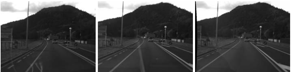
Fig. 1. One time frame of image sequences taken with three cameras (called: third, left, and right camera - from left to right) installed in HAKA1, test vehicle of the .enpeda.. project. Note the reflections on the windscreen, and differences in lightness (e.g., image of right camera is brighter than the other two). Left and right views are rectified.
