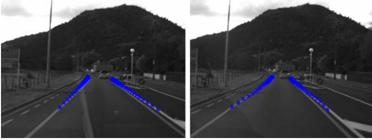
Fig. 8. Detected lanes (for left and right image as shown in Figure 11), illustrating robustness of the technique (i.e., independence of camera position)
