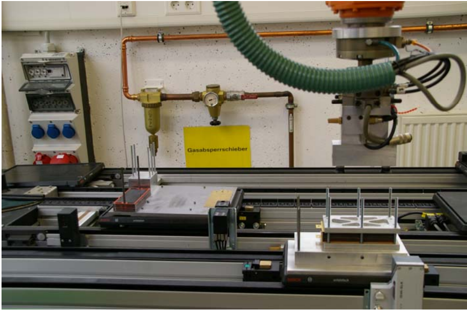
Fig. 7. Robot with gripper-change-system an vacuum-gripper
