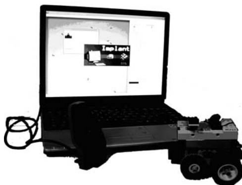
Fig. 3. The transfer of the control system (an Artificial Neural Network) from the simulator BreedBot to the real Lego MindStorms robot, through the infrared port
