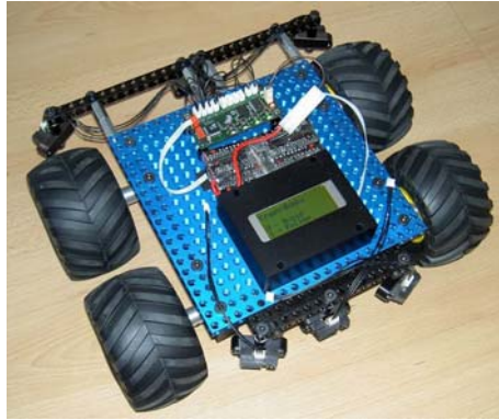
Fig. 11. Offroad robot with differential drive
