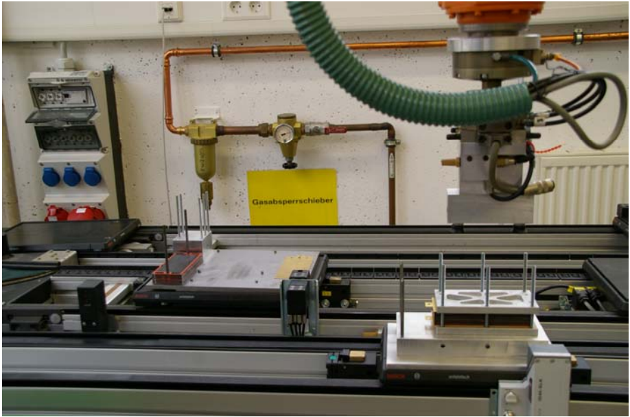
Fig. 7. Robot with gripper-change-system an vacuum-gripper
