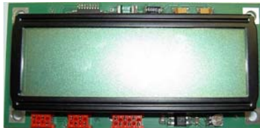
Fig. 8. “LCD display board”: expansion board with LCD display
