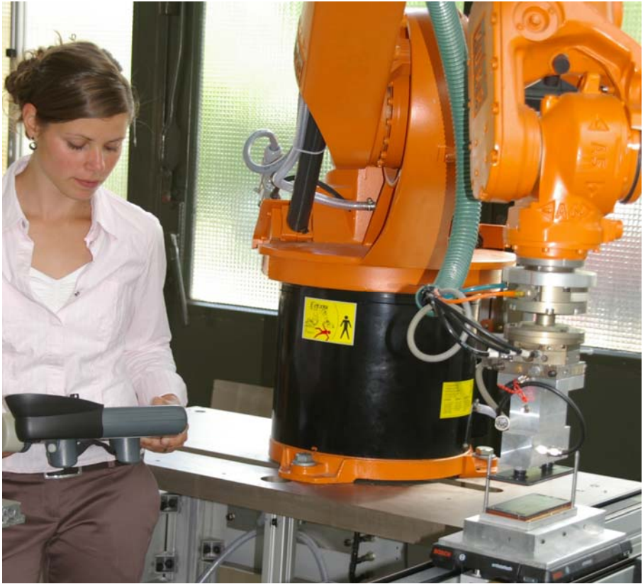
Fig. 8. Programming (teaching) of a Kuka robot
