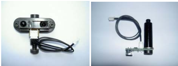
Fig. 5. Left: Bearing Sharp IR distance sensor. Right: Bearing for a CNY70 line sensor.
