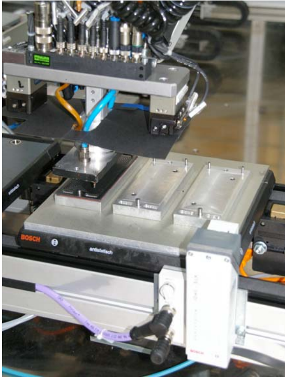
Fig. 4. Carrier in the assembly station with 3 storage places
