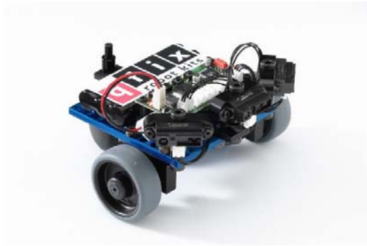
Fig. 1. Crash-Bobby, a differential drive robot with two driven wheels and three IR distance sensors
