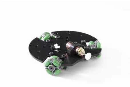
Fig. 12. Omnidrive platform with three omnidirectional wheels
