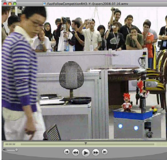
Fig. 7. Our robot RH3-Y follows our team member Illkyun Jeon at speed of up to 1m/s through the “Home” at Robocup competition 2008 in Suzhou, China, successfully crossing next another team
