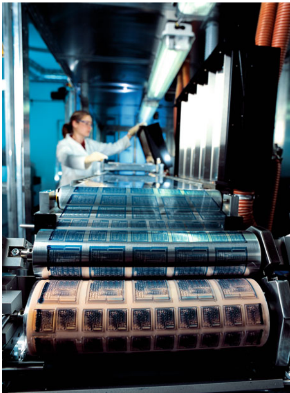
Fig. 4 Organic electronics produced in a roll-to-roll printing process (PolyIC Press Picture. © PolyIC 2006)
