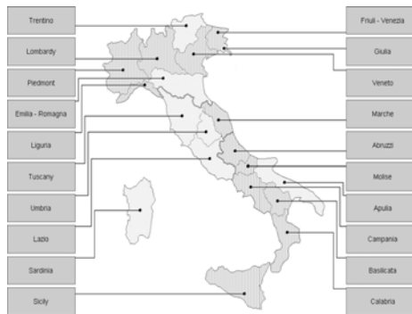
Fig. 4. Minimal leader lengths for labels on two opposite sides of the rectangle
