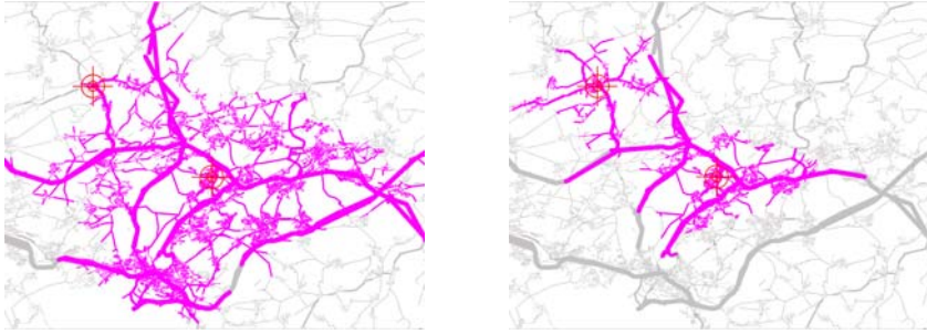
Fig. 1. The search space of Dijkstra's algorithm on a road network, for a given source and target. Left: the original algorithm. Right: its bidirectional version.
