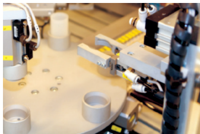
Fig. 10.2. An automatic system to fill bottles
